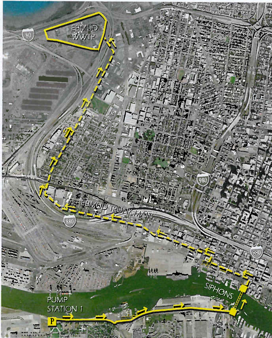
Figure 6-2: Existing Off-Site Sanitary Sewer Systems
