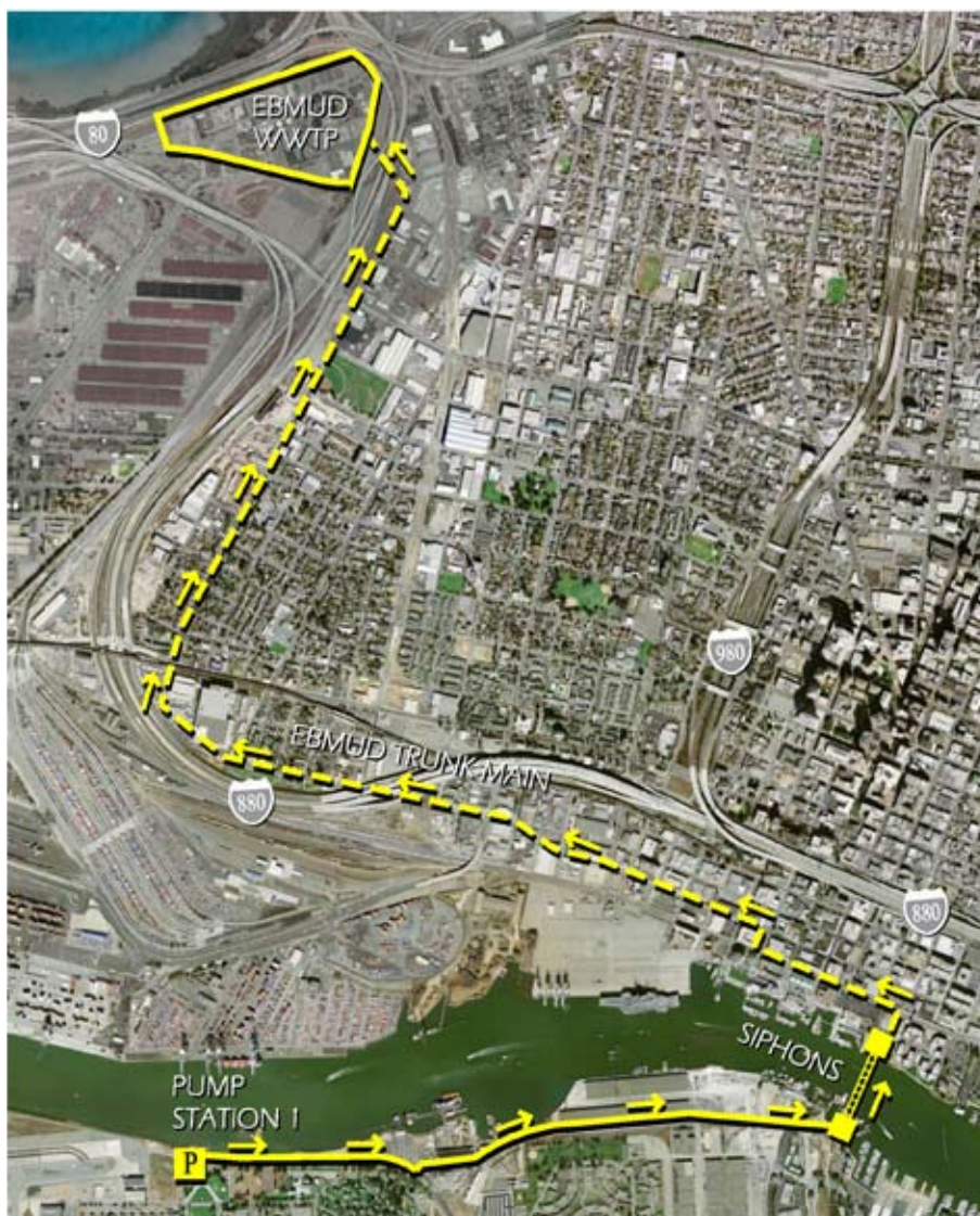
Figure 6-2: Existing Off-Site Sanitary Sewer Systems
